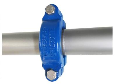
The HYDROMINE™ HMP\_TE pipe coupling can be installed in a system where pipes hang on chains, parrot swings or are U-Bolted down onto pipe supports. Pipes should be anchored before and after every change of direction. The full range of HYDROMINE™ LFC\_1B valves, LFC\_8 expansion joints and LFC\_7 energy dissipator can be manufactured with HYDROMINE™ HMP TE coupling end connections.
